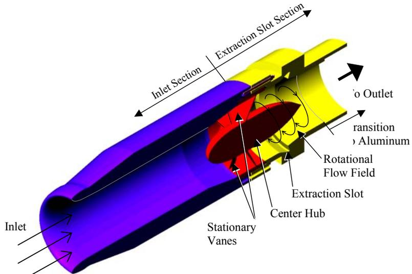
**Figure 2. Interior schematic of the cloud collector.**
