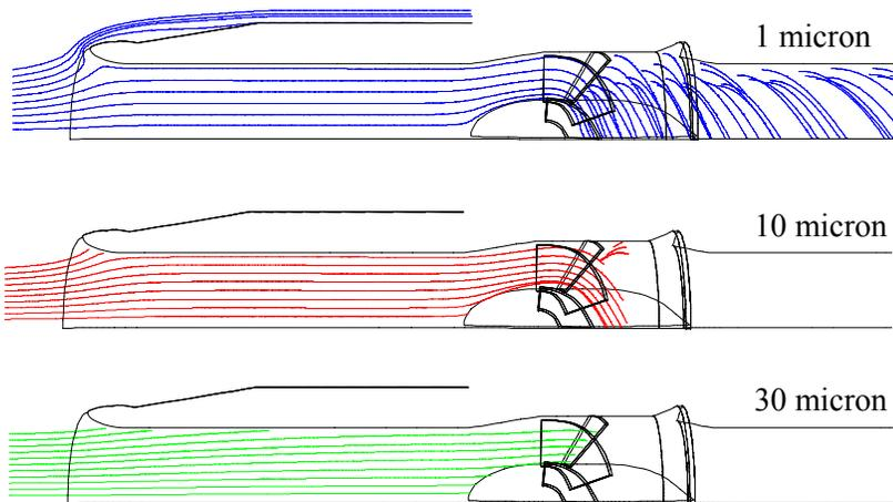
**Figure 3. CFD trajectories for a) 1  $\mu\text{m}$ , b) 10  $\mu\text{m}$ , and c) 30  $\mu\text{m}$  diameter drops.**
