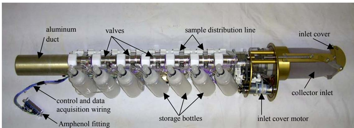
**Figure 1. Picture of the final axial-flow cloud water collector shown outside of the modified PMS canister.**
