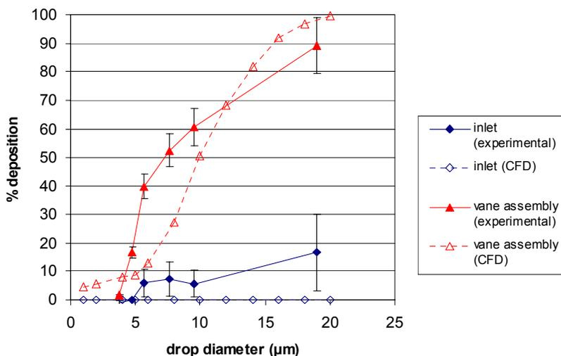
**Figure 5. Experimental and modeled drop deposition in the axial-flow collector inlet and on the vane assembly.**
