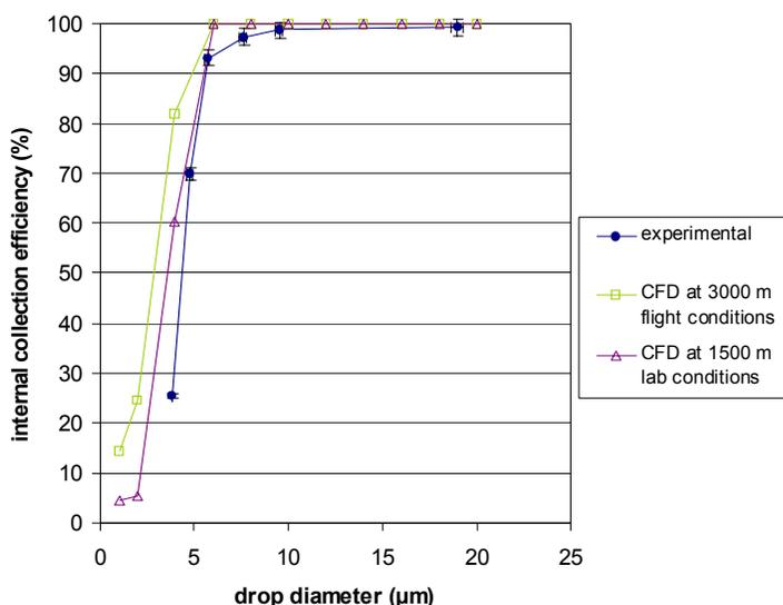
**Figure 4. Experimental and modeled internal collection efficiency curves for the axial-flow cyclone cloud collector.**
